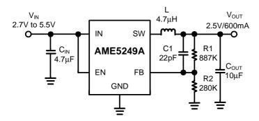
Figure 6. AME5249A with 2.5V Output
