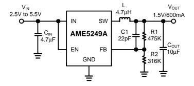
Figure 5. AME5249A with 1.5V Output
