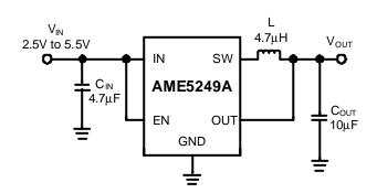
Figure 1. Fixed Voltage Regulator
