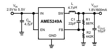
Figure 2. Adjustable Voltage Regulator
