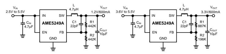
Figure 4. AME5249A with 1.2V Output
